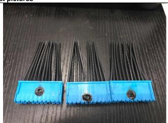
Visual examination picture of post-test at 750 °C (1-2364737-1)
