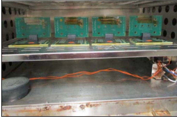
Figure 6 – Typical Humidity Test Setup
