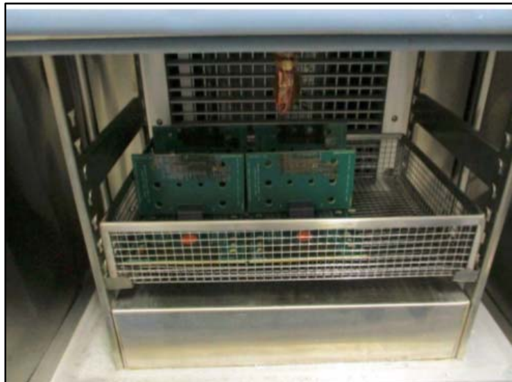
Figure 5 – Typical Thermal Shock Test Setup
