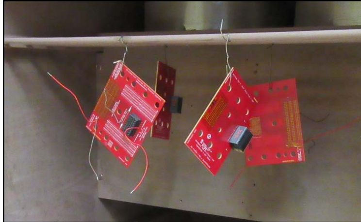
Figure 9 – Dust Contamination Setup
