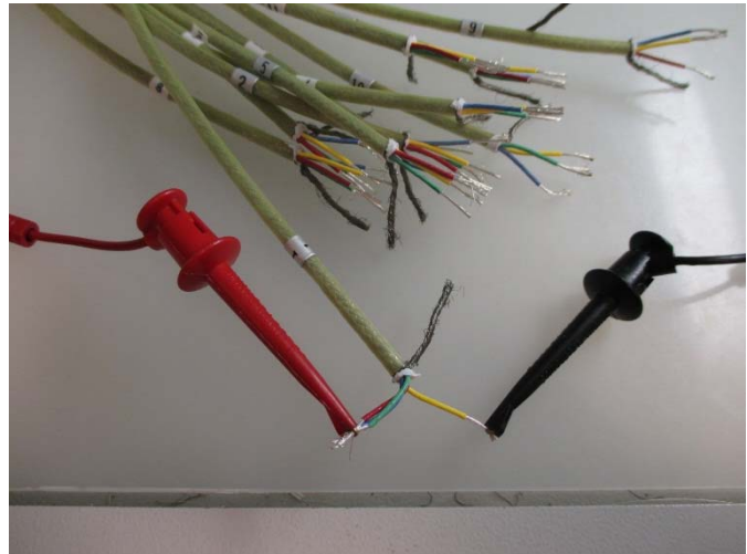
Figure 2 – Initial Dielectric Withstanding Voltage / Insulation Resistance Test Setup
