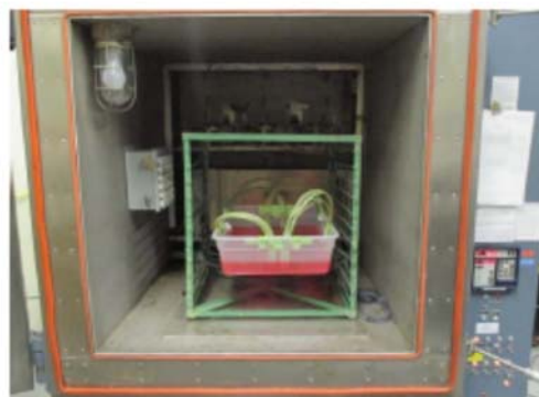
Figure 2 – Altitude Chamber Setup
