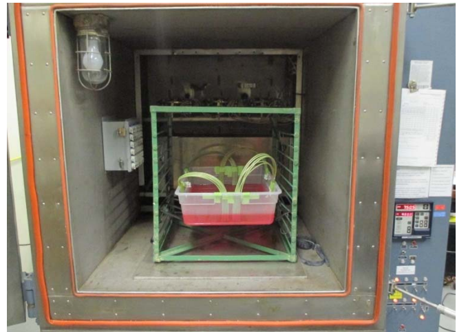
Figure 6 – Altitude Immersion Test Setup
