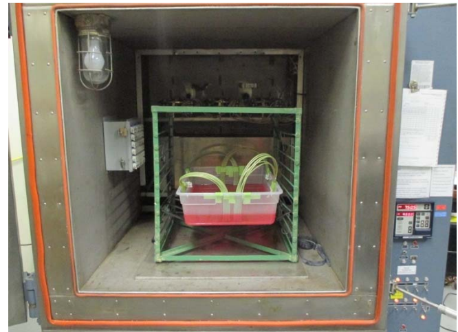
Figure 6 – Altitude Immersion Test Setup
