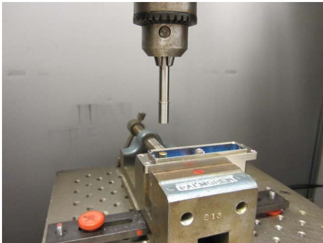
Figure 7 – Contact Retention Test Setup
