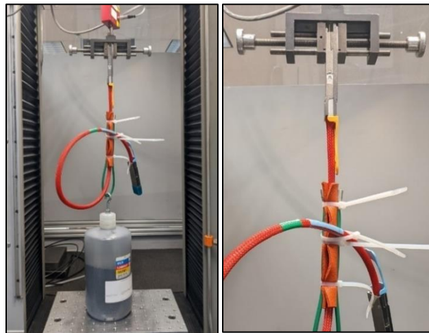
Figure 5 – Typical Axial Cable Retention Test Setup
