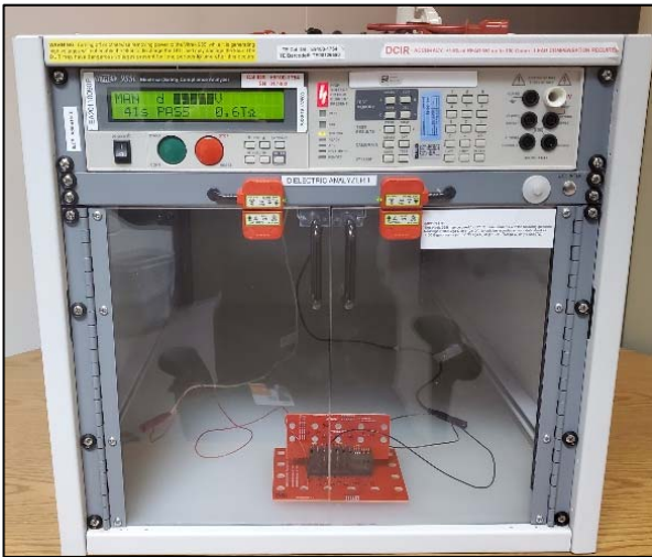
Figure 5 – Insulation Resistance Measurements at Ambient Condition
