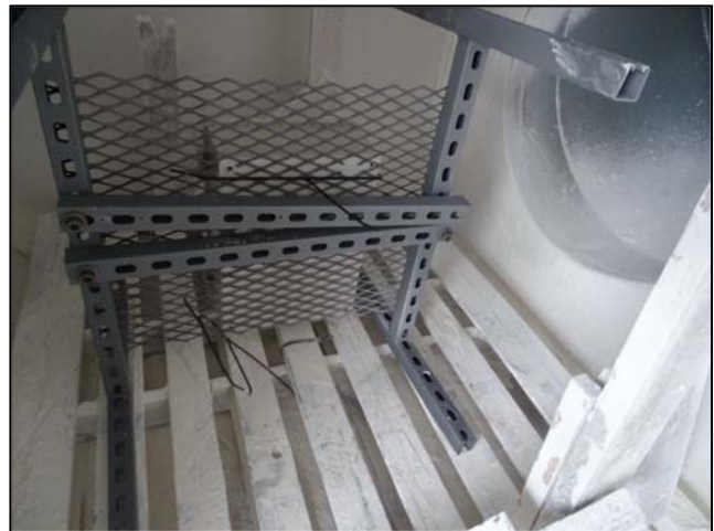
Figure 28 – Enclosure in Dust Chamber Orientation 2
