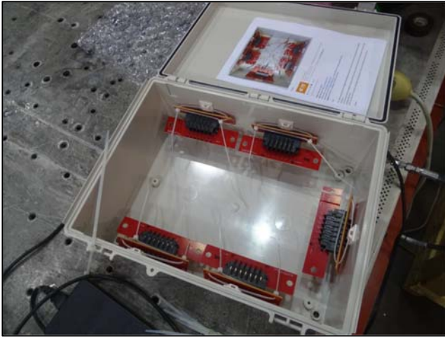
Figure 25 – Specimens Secured In Simulated Plug-In Unit Enclosure
