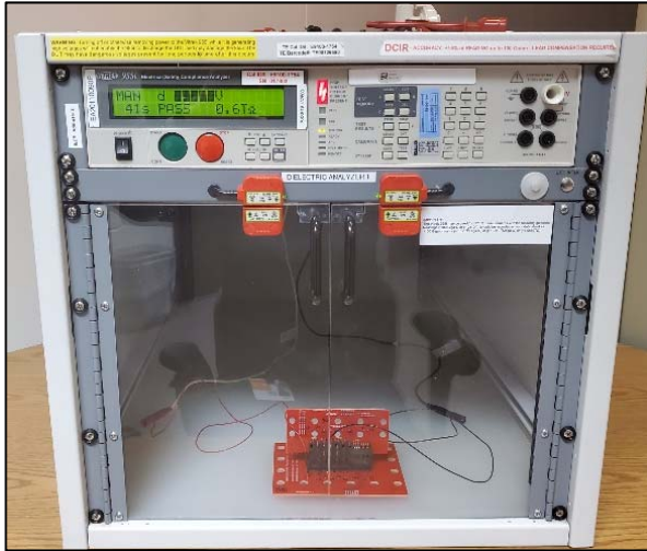
Figure 10 – Dielectric Withstanding Voltage Testing at Ambient Condition
