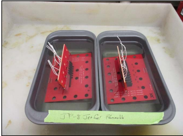
Figure 31 – Fluid Contamination Immersion
