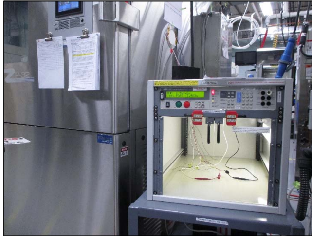
Figure 7 – Insulation Resistance Measurements at High Humidity
