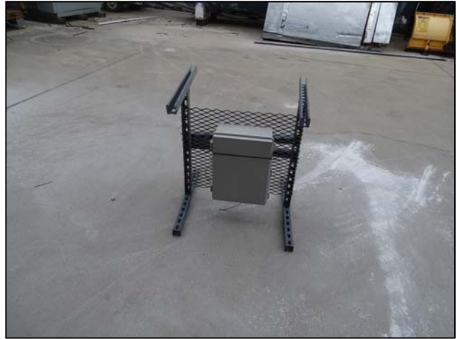
Figure 26 – Simulated Plug-In Unit Enclosure Secured to Test Frame
