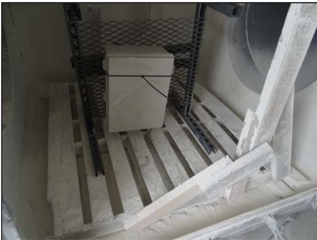
Figure 27 – Enclosure In Dust Chamber Orientation 1
