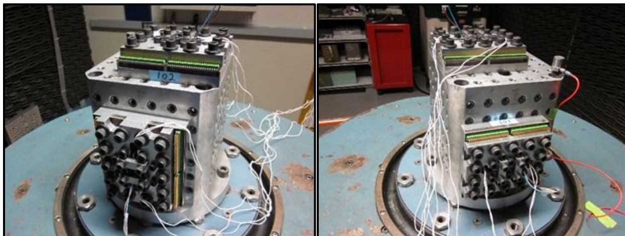
Figure 8 – Vibration/Mechanical Shock Test Setup
