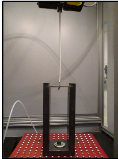
Figure 9 – Typical Wire Crimp Tensile Strength Setup
