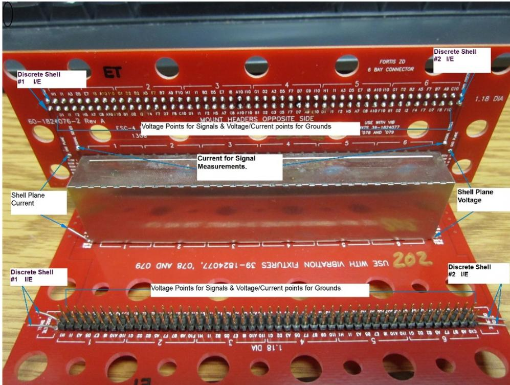
Figure 3 – Typical Low Level Contact Resistance Measurement Points
