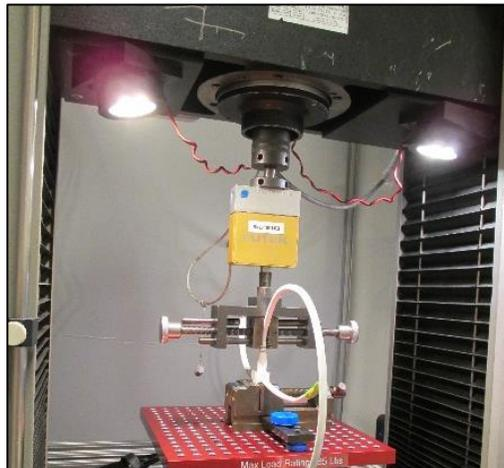
Figure 9 – Unmating Force Test Setup
