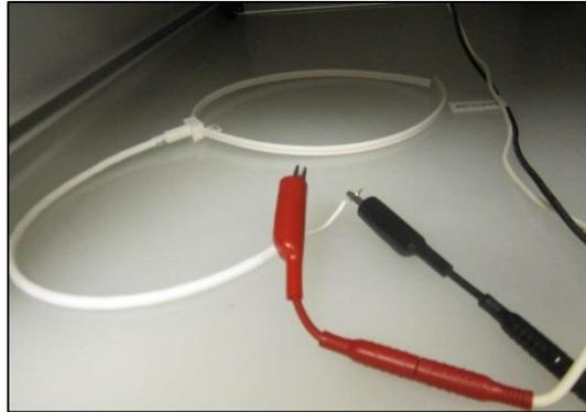
Figure 3 – IR and DWV Test Setup - Adjacent Contacts
