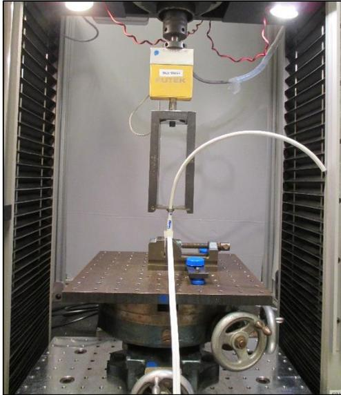
Figure 7 – Mating Force Test Setup
