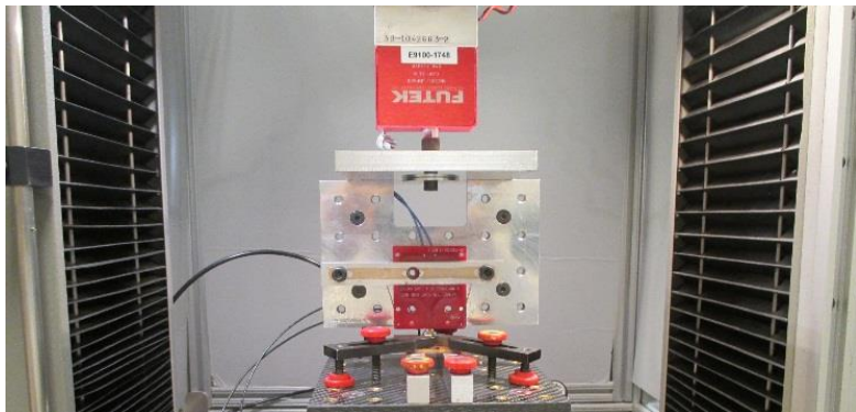
Figure 11 - Unmating Test Setup
