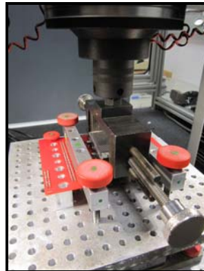
Figure 8 – Press Fit Extraction Force Test Setup
