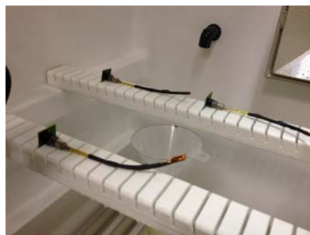
Figure 17 – Salt Spray Test Setup
