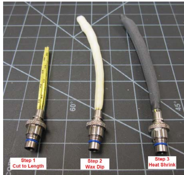
Figure 11 – Hydrostatic Water Immersion Specimen Preparation
