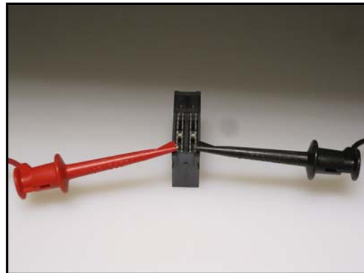
Figure 5- Left to Right Withstand Voltage Test setup
