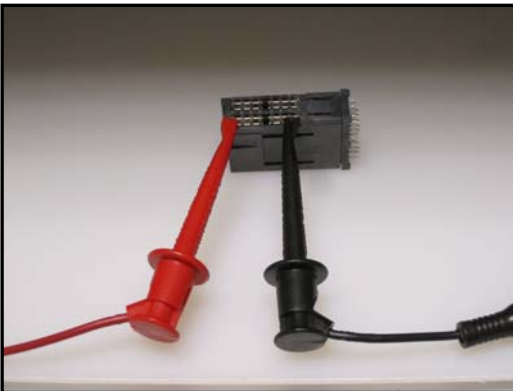
Figure 4- Front to Back Withstand Voltage test setup
