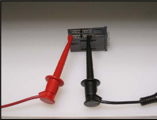
Figure 2- Front to Back IR test setup
