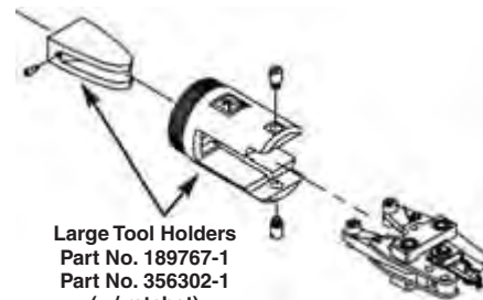
Platform Die Set Adapter Part No. 679992-1
