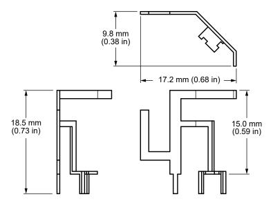
Figure 1. ANT-W63-MSA-TH1 Antenna Dimensions
