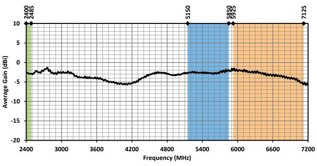
Figure 6. ANT-W63-MSA-TH1 Average Gain with Frequency Band Highlights
