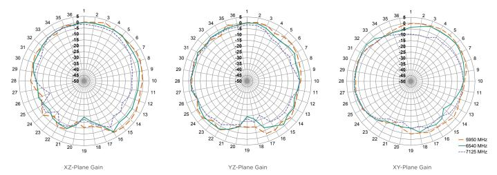
Figure 8. ANT-W63-MSA-TH1 Antenna Radiation Patterns
