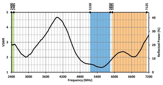
Figure 3. ANT-W63-MSA-TH1 Antenna VSWR with Frequency Band Highlights
