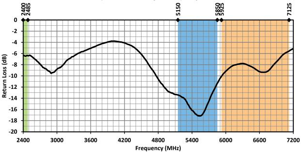
Figure 4. ANT-W63-MSA-TH1 Return Loss with Frequency Band Highlights
