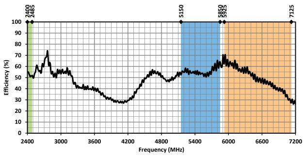
Figure 7. ANT-W63-MSA-TH1 Radiation Efficiency with Frequency Band Highlights
