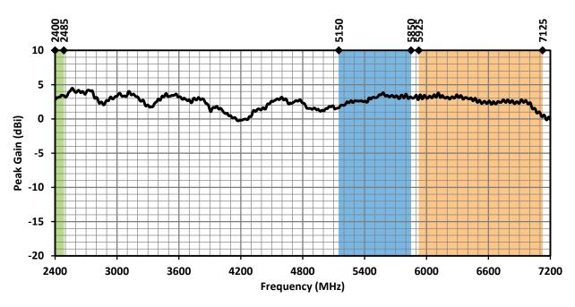
Figure 5. ANT-W63-MSA-TH1 Antenna Peak Gain with Frequency Band Highlights
