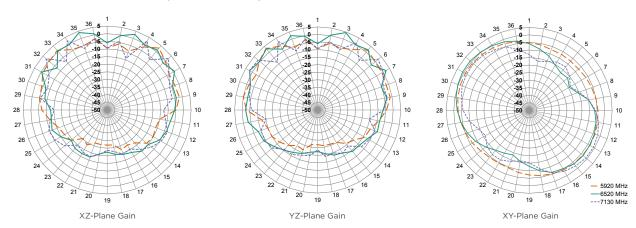
Figure 16. Radiation Patterns for the ANT-W63-IPW2-NP Antenna, Center of Ground Plane
