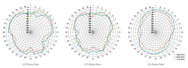
Figure 9. ANT-W63-IPW2-NP Antenna Radiation Patterns, Free Space
