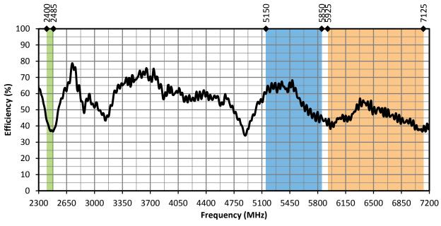
Figure 15. ANT-W63-IPW2-NP Antenna Radiation Efficiency, Center of Ground Plane
