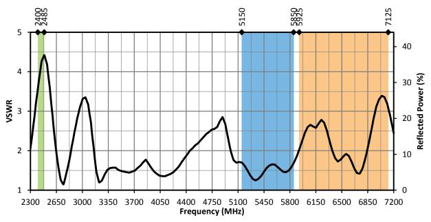
Figure 11. ANT-W63-IPW2-NP Antenna VSWR, Center of Ground Plane
