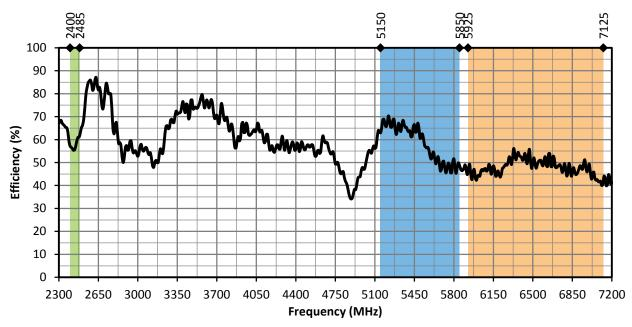
Figure 8. ANT-W63-IPW2-NP Series Antenna Radiation Efficiency, Free Space
