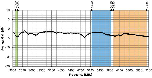
Figure 14. ANT-W63-IPW2-NP Antenna Average Gain, Center of Ground Plane
