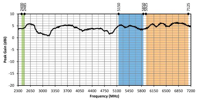
Figure 13. ANT-W63-IPW2-NP Antenna Peak Gain, Center of Ground Plane
