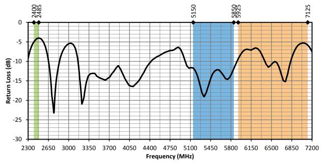
Figure 12. ANT-W63-IPW2-NP Antenna Return Loss, Center of Ground Plane
