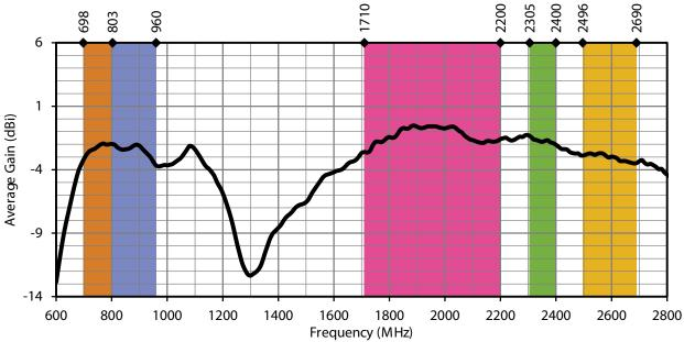
Figure 4. SP610 Average Gain with Frequency Band Highlights
