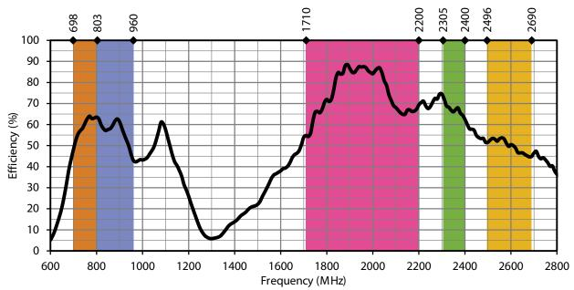
Figure 5. SP610 Radiation Efficiency with Frequency Band Highlights
