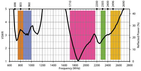
Figure 1. SP610 VSWR with Frequency Band Highlights
