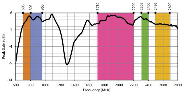
Figure 3. SP610 Peak Gain with Frequency Band Highlights
