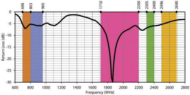
Figure 2. SP610 Return Loss with Frequency Band Highlights
