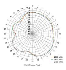
Figure 8. Radiation Patterns for the SP610 Antenna
