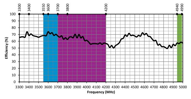
Figure 15. 5GMWP1 Antenna Efficiency, Edge-Bent
