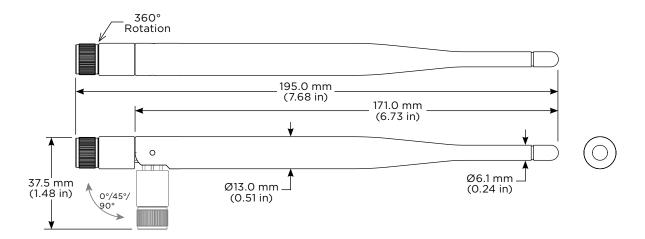
Figure 1. 5GMWP1 Antenna Dimensions
