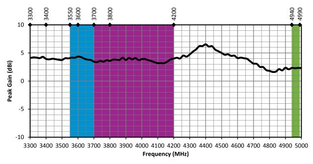
Figure 13. 5GMWP1 Peak Gain, Edge-Bent
