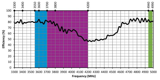
Figure 8. 5GMWP1 Antenna Efficiency, Straight
