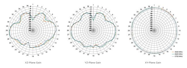
Figure 16. Antenna Radiation Patterns for the 5GMWP1, on Edge of Ground Plane, Bent at 90 Degrees
