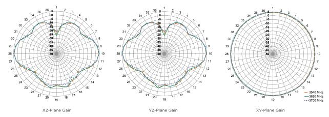
Figure 9. Antenna Radiation Patterns for the 5GMWP1, Straight
