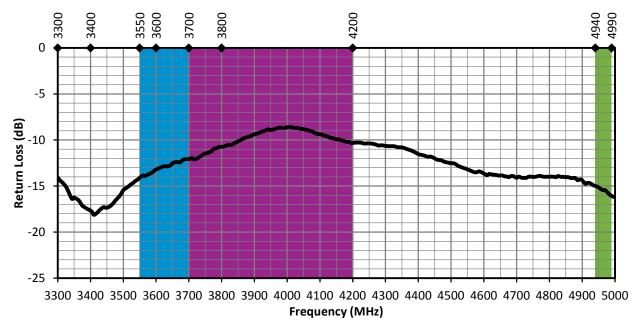
Figure 12. 5GMWP1 Return Loss, Edge-Bent
