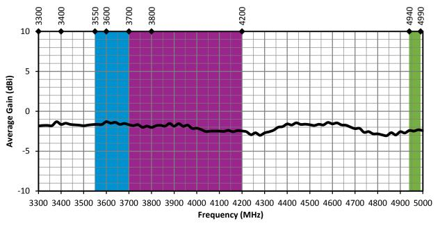
Figure 14. 5GMWP1 Average Gain, Edge-Bent
