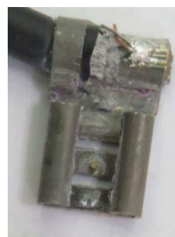
Figure 2: Post-Tin Brass Terminals
