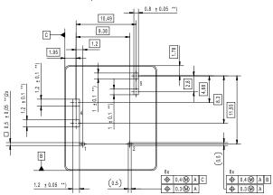
Remark: Positional tolerances according to DIN EN ISO 5458
