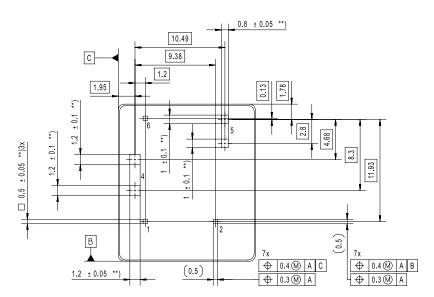
Remark: Positional tolerances according to DIN EN ISO 5458 \*\*) without tinning (hot dip)
