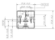
**Dimensions** (special cover with notches -V23136-A0001-X083)
