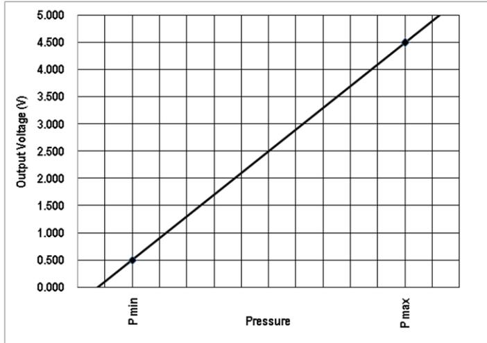
$$\text{Output Voltage} = \left[ \frac{0.8}{(P_{\text{max}} - P_{\text{min}})} \times (\text{Pressure applied} - P_{\text{min}}) + 0.1 \right] \times \text{Supply Voltage}$$
