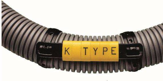
K-Type markers are used to identify wire bundles, cables, pipes and conduits. The oval shaped profile has been designed to allow markers to be accurately positioned onto a carrier strip. The marker and carrier strip assembly is attached to the substrate using cable ties. K-Type markers are ideal for post termination applications or where retrofitting is required.
