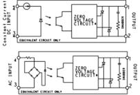
\* Random Turn-on Units have a Random Turn-on circuit instead of Zero Voltage Circuit
