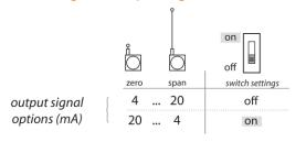
The SR1M leaves the factory set with a 4...20 mA full scale output signal. The signal can be reversed (see illustration) by simply changing a dipswitch located on the controller board.
