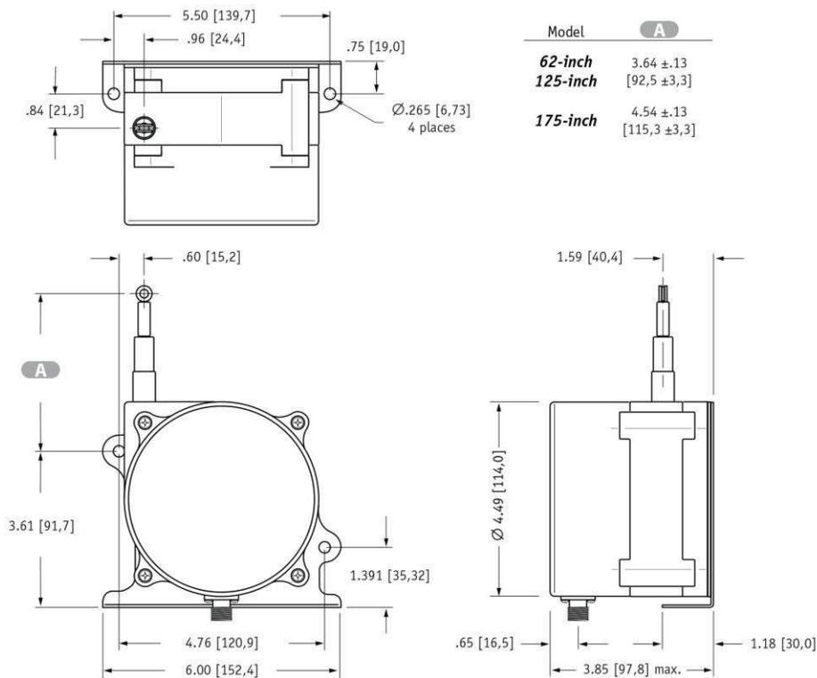
**Fig. 3 – “Down” Cable Exit Direction:**
