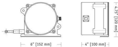
SR1A is a rugged, low-cost, high performance string pot built for wet environments and outdoor applications. Originally designed for off-road construction equipment, the SR1A is the perfect low-cost solution for OEM and stocking distributors.
