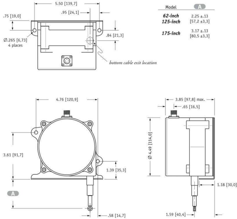
**Fig. 4 – “Rear” Cable Exit Direction:**
