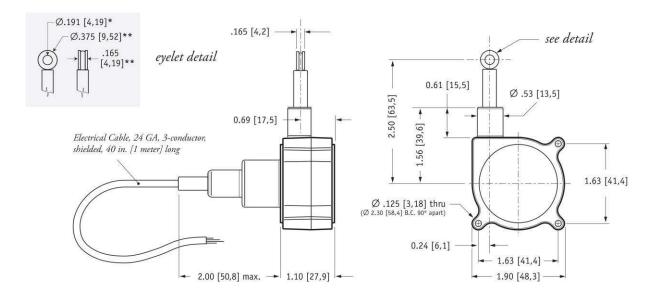
DIMENSIONS ARE IN INCHES [MM] tolerances are 0.04 IN. [1,0 MM] unless otherwise noted.
