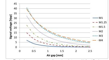
Typical sensor output voltage (peak-to-peak) for 15m/s
