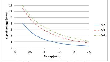
Typical sensor output voltage (rms) for 15m/s
