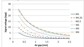
Typical sensor output voltage (peak-to-peak) for 15m/s
