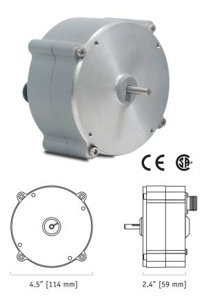
The RT9420 provides rotational position feedback via 4...20 mA current loop signal. This device combines the superb linearity and resolution of a plastic-hybrid potentiometer and the durability of our 4...20mA circuit to provide an accurate and reliable electrical signal. Additionally the zero and span settings are adjustable through access holes in the housing.
