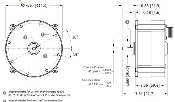
M4 x 4,5 mm @ 90° apart on a 105,4 mm dia. BC (4 places) 3 reference mark full counter-clockwise position - align mark on shaft to mark on face for start of measurement range
