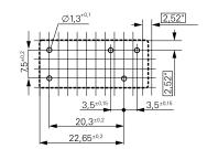
\*) With the recommended PCB hole sizes a grid pattern from 2.5mm to 2.54mm can be used.
