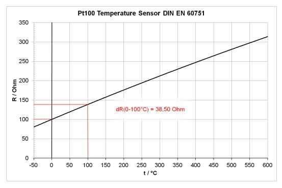
Figure 1: Resistance characteristics (For Pt1000 use for Resistance Values Scale a Nominal Resistance Factor 10)
