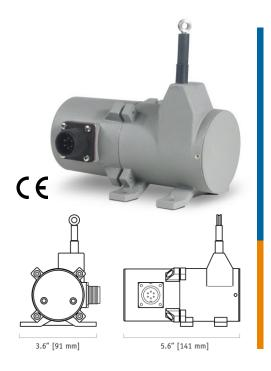
The PT8510 can operate from an unregulated 14.5 to 40 VDC power supply while providing an output signal that is proportional to the linear movement of its measuring cable. The PT8510 has a maximum measurement range up to 60" and has 4 output signal options to choose from: 0...10, 0...5, -10...+10 and -5...+5 Vdc.
