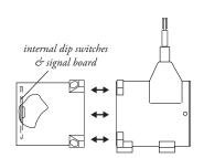
To gain access to the signal board, remove four Allen-Head Screws and remove rear cover.
