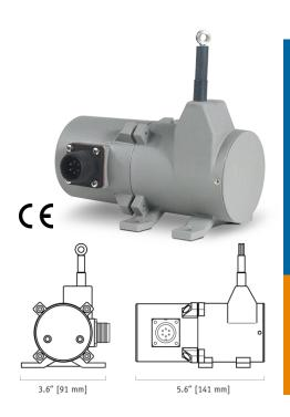
The PT8101, using a high cycle plastic-hybrid potentiometer, operates with any basic panel meter or programmable controller in factories and harsh environments requiring linear position measurements in ranges up to 60".
