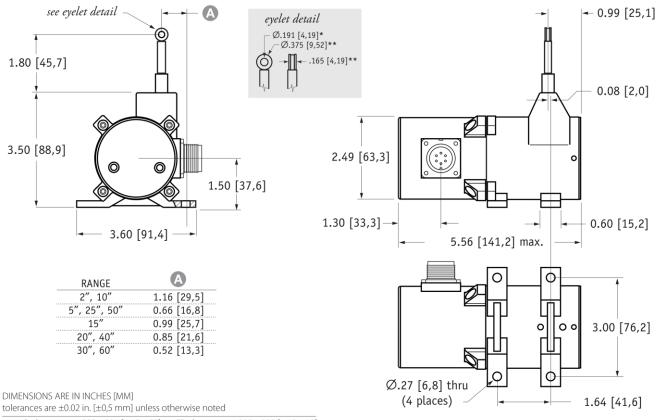
note: \*tolerance = +.005 -.001 [+.13 -.03] \*\*tolerance = +.005 -.005 [+.13 -.13]
