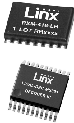
Figure 9: Receiver and Decoder
