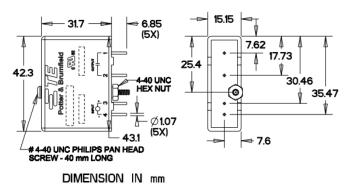
Note : Extra nut and washer will be provided on the screw, which will goes under PCB to fix the relay. Hex Nut S= 6.35 (width across flats), Thickness = 2.40; Washer = OD :  $\Phi$ 485±0.25, ID :  $\Phi$ 2.75±0.15, Thickness : 0.55
