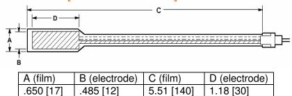
Connector provides two 0.025" square pins on 0.1" spacing and will mate with a wide range of FFC (flexible flat cable) receptacles.
