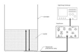
Liquid presence/absence in pipe or cylindrical vessel (high S/N ratio)
