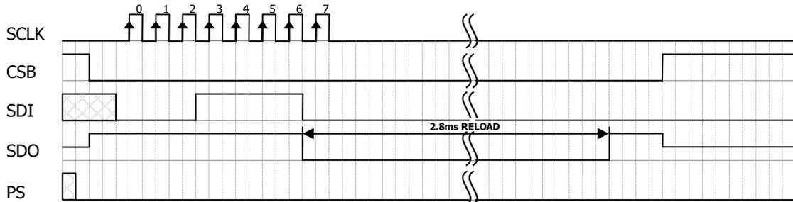
Figure 9: Reset command sequence SPI mode 0
