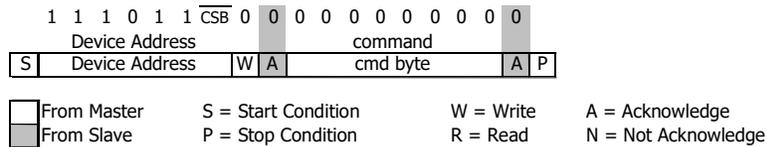
Figure 5: I<sup>2</sup>C ADC read sequence
