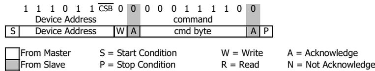
Figure 3: I<sup>2</sup>C Reset Command
