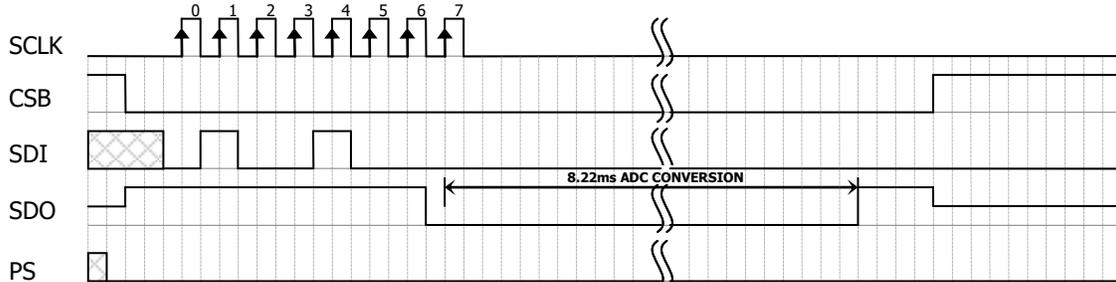
Figure 11: Conversion out sequence, Typ=d1, OSR = 4096
