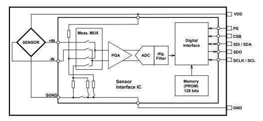
Figure 1: Block diagram of MS5803-01BA
