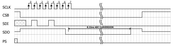
Figure 11: Conversion out sequence, Typ=d1, OSR = 4096
