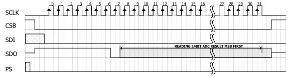
Figure 12: ADC Read sequence
