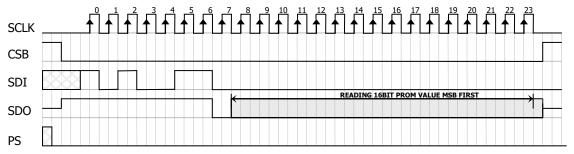
Figure 13: PROM Read sequence, address = 011 (Coefficient 3).
