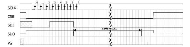
Figure 10: Reset command sequence SPI mode 3
