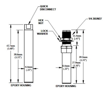
Figure 2: ML series elements sensors
