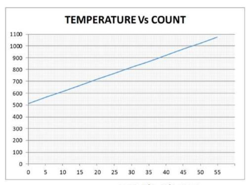
OUTPUT (DECIMAL COUNTS)=  $\frac{(\text{OUTPUT}^{\circ}\text{C}+50 ^{\circ}\text{C})\text{X}2048}{150 ^{\circ}\text{C}-(-50 ^{\circ}\text{C})}$
