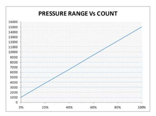
OUTPUT (DECIMAL COUNTS)=  $\frac{15000-1000}{\text{Pmax-Pmin}}X \quad (\text{Papplied-Pmin})+1000$
