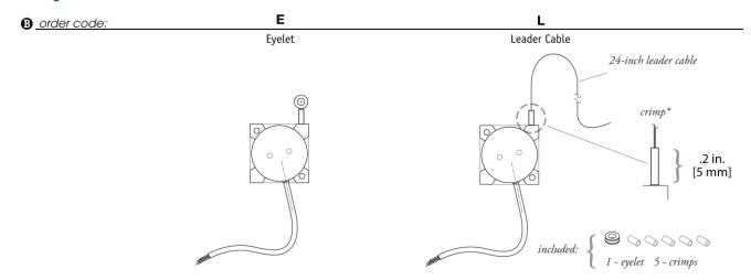
\*note: crimped stop prevents leader cable from retracting into sensor body
