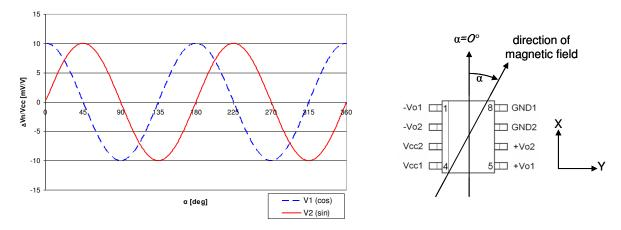
Figure 2: Characteristic curves for KMT37
