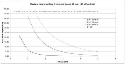
Figure 1: Maximal output voltage of the sensor Legend:
