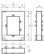
A range of split core current transformers that offers a cost effective and efficient method by which the current can be measured without the need to break the conductor, thereby reducing installation and commissioning time.
