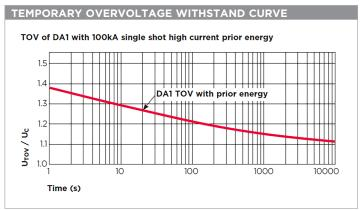
U<sub>TOV</sub> = temporary overvoltage withstand
